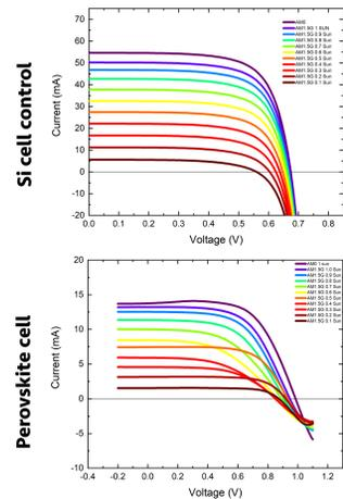
A linear relationship between I<sub>sc</sub> and light intensity was observed in the IV plots of the Si control cell. In contrast, the perovskite sample showed saturation effects at higher intensities and an unexpected spike in power at 0.5 and 0.2 suns.
