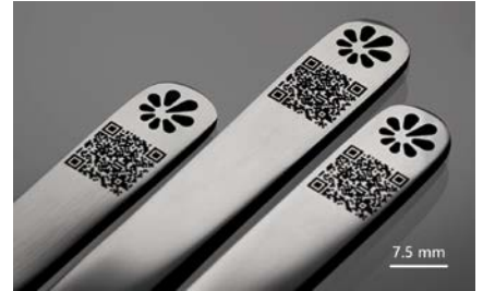
Black marking of tweezers. Courtesy of FTMC.
